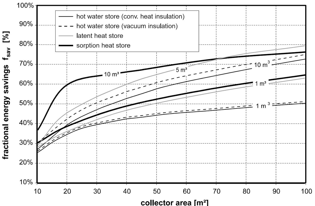
**Figure 1:** Fractional energy savings for different store technologies and store volumes (plus 750 litres for the “conventional” combistore) as a function of the collector area (flat plate collector)
