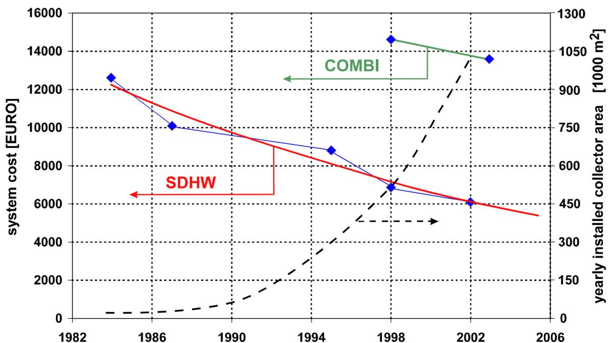
**Figure 3:** Development of average costs for thermal solar systems (incl. VAT and installation); Source: Stiftung Warentest
