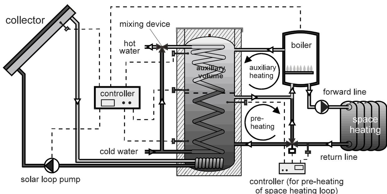
**Figure 2a:** Schematic design of a combisystem with space heating loop operated in pre-heating mode
