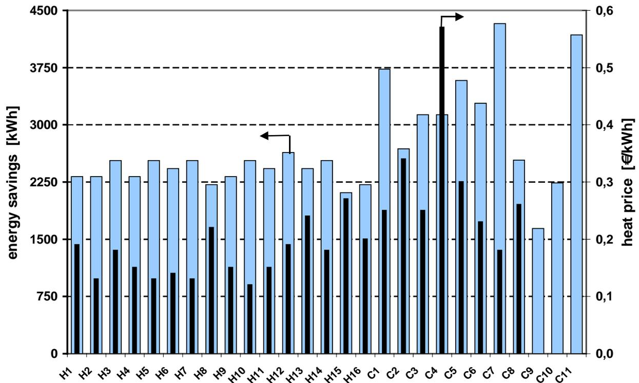
Figure 4: Energy savings and heat price of solar domestic hot water systems (H) and solar combisystems (C)
