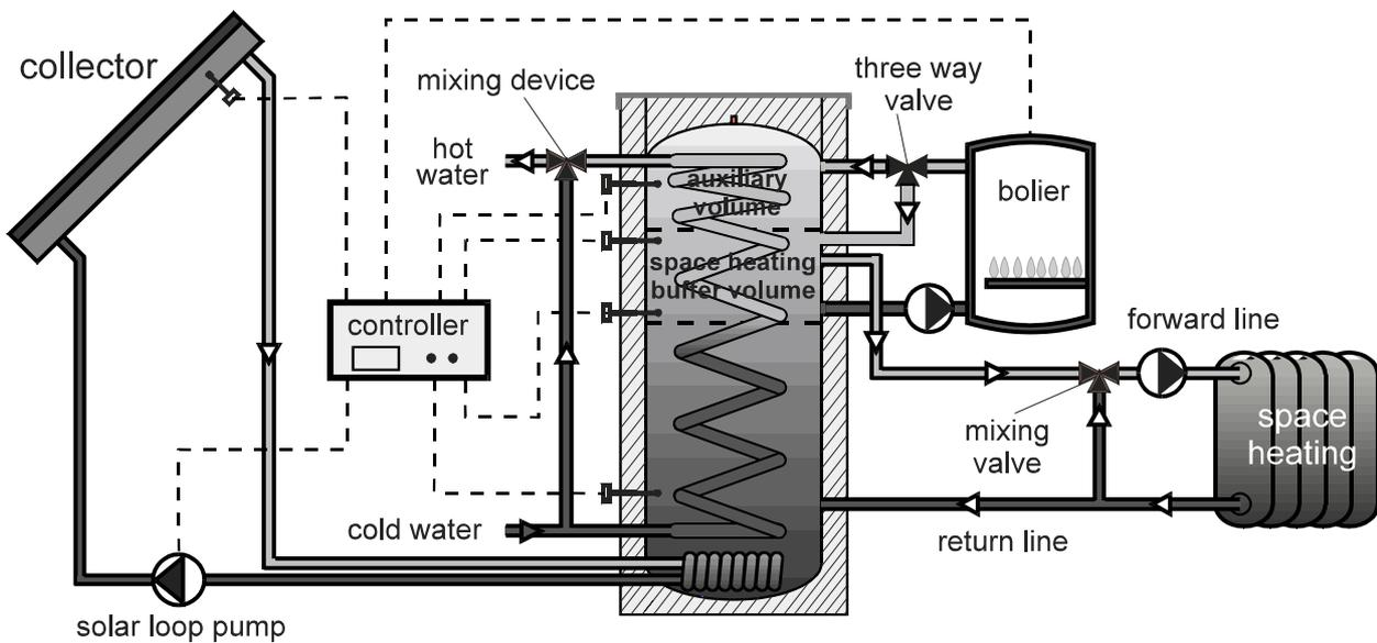
**Figure 2b:** Schematic design of a combisystem using the combistore as a buffer store
