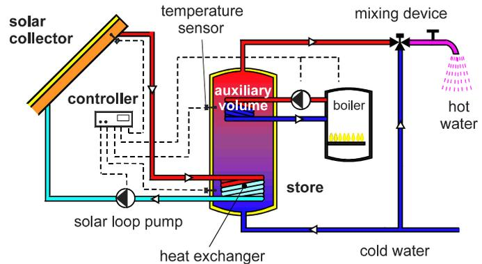
**Figure 1:** Schematic setup of standard German solar domestic hot water system
