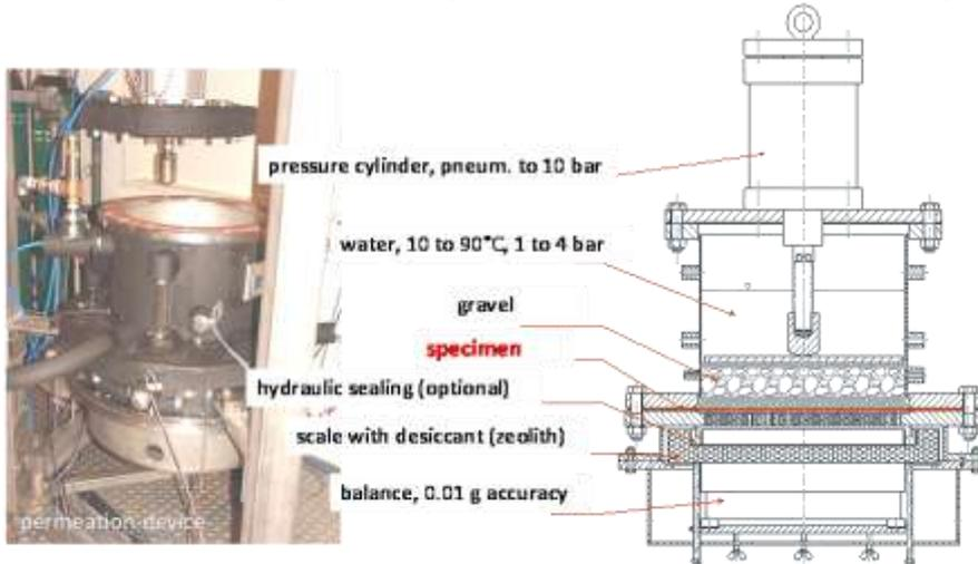
Figure 3. Photo and sketch of the permeation measurement device
