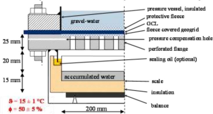
Figure 4: Schematic configuration of the measurement device (non-scale)
