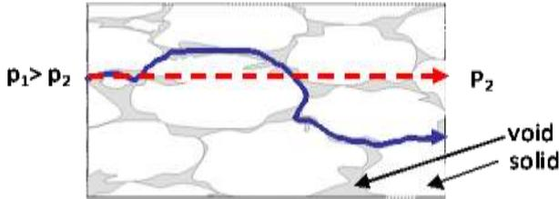
**Figure 2.** Water vapour diffusion through a porous medium, water vapour resistance as extra path length
