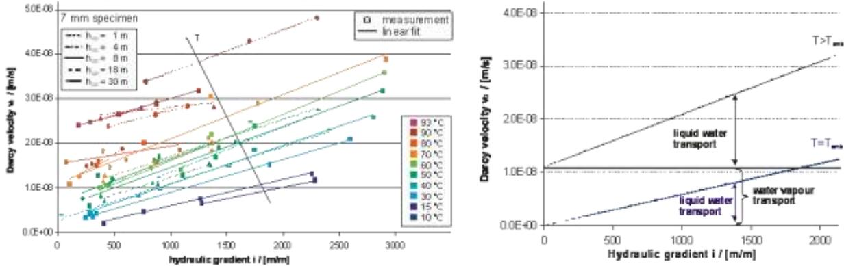
**Figure 6.** left: measured Darcy velocity as a function of the hydraulic gradient ( $i=\Delta H/d$ ) with the height of the gravel cover ( $h_{GW}$ ) and the temperature (T) as parameter, right: schematic pure liquid water permeation rate as a function of hydraulic gradient and superimposed water vapour transport
