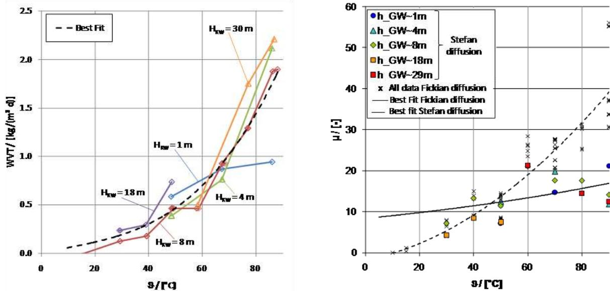
**Figure 8.** Water vapour transmission WVT as a function of temperature  $\theta$ ; Water vapour diffusion resistance factor  $\mu$  determined according to the Fickian Law (x) and according to Stefan diffusion (filled marker)
