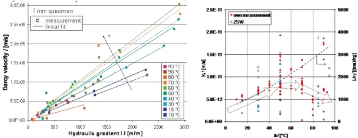
**Figure 7.** left: pure liquid water permeation rate in a temperature range from 10 °C to 93 °C as a function of the hydraulic gradient ( $i=\Delta H/d$ ) with the height of the gravel cover ( $h_{GW}$ ) as parameter, right: reciprocal dynamic viscosity as well as measured hydraulic conductivity as a function of temperature, comparison of own measurements with measured data from ZSW.
