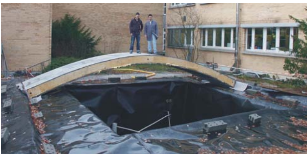
Fig. 2: Sandwich element mounted on the pit, static (human) load test
