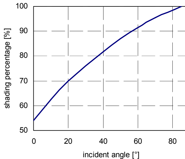
Fig.3: shading percentage as a function of incidence angle
